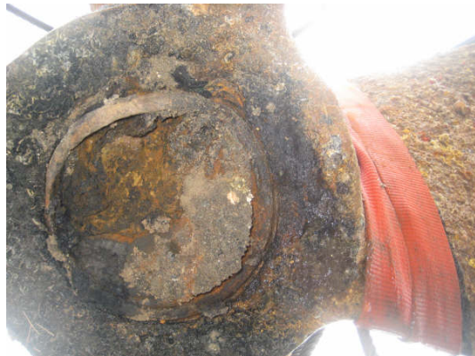
MISC. PHOTO: Close up of the hub of the propeller and the broken shaft
